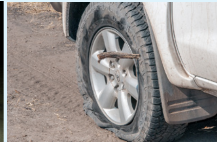
Deflating the tyres to a third or more of the normal pressure is a huge assistance for sand driving but makes the tyre side walls much more prone to punctures (Namibia)
