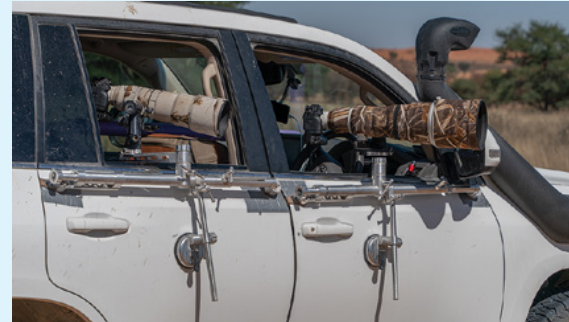
Close-up of the commercially available door mounted camera support systems attached to the Landcruiser (Etosha, Namibia)
